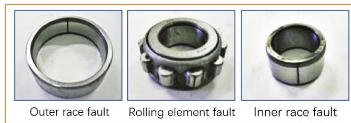
Fig. 7. Images of different types of bearing faults
