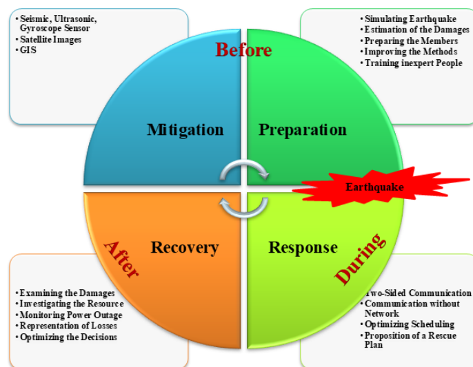
Fig. 1. Effect of IoT on earthquake disaster mitigation
