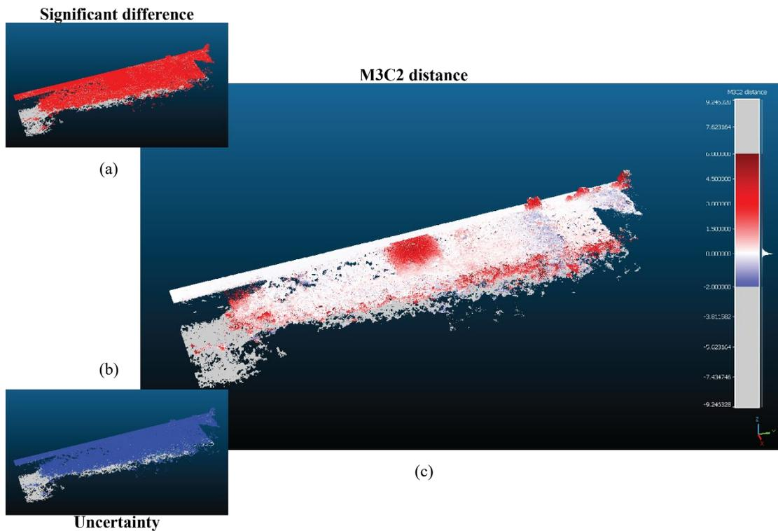
Fig. 4. Dense point clouds comparison for ISI-1: 2020-02-10, and ISI-3: 2021-02-10: (a) Significant difference between the two point clouds, (b) Uncertainty when comparing the two point clouds, and (c) Calculated M3C2 distance between the two point clouds indicating the areas of identified variations
