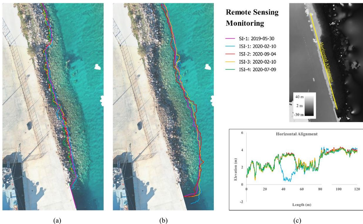
**Fig. 5.** (a) Waterline, (b) toe line, and (c) an indicative longitudinal profile for the rubble mound structure of the ferry domestic domain at Lavrio port as produced by the analysis of the two multimodal data, i.e., satellite imagery (SI-1) and aerial imagery (ISI-1, ISI-2, ISI-3, and ISI-4)
