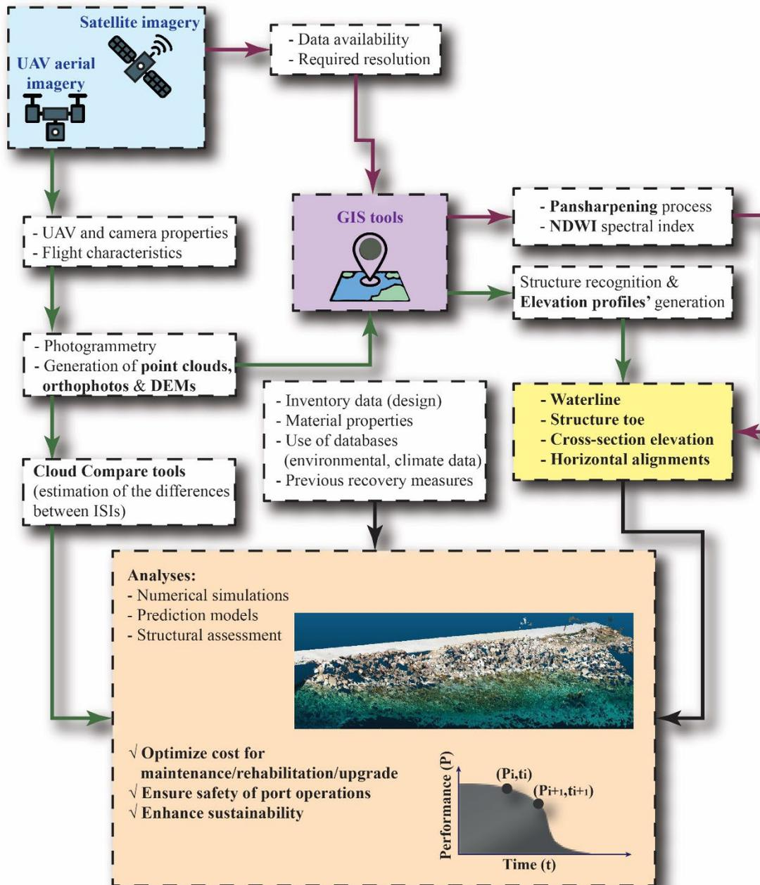
**Fig. 1.** Multimodal RS framework for port infrastructure monitoring towards assessing the structural performance of rubble mound structures
