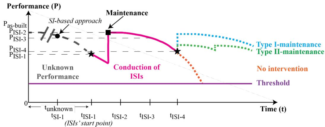
**Fig. 7.** Life-Cycle Performance for the rubble mound structure at the domestic ferry domain of Lavrio port considering the applied RS monitoring framework
