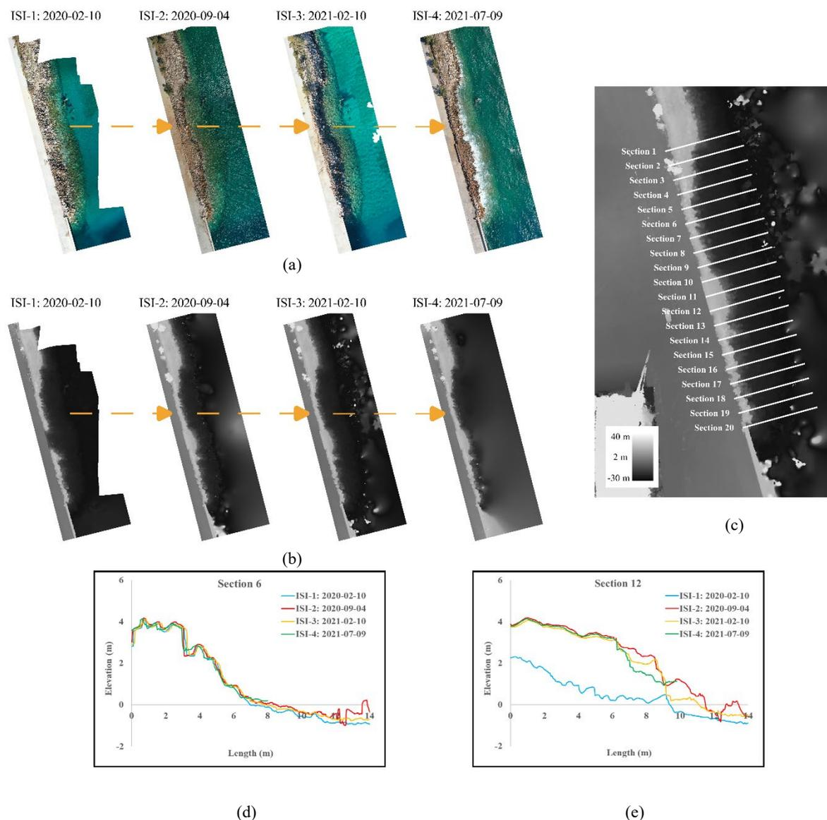
**Fig. 6.** Elevation changes of the armour layer of the rubble mound structure of the domestic ferry domain at Lavrio port: (a) change detection in the orthophotos of the four (4) UAV-based in situ inspections, (b) change detection in the DEMs of the four (4) UAV-based in situ inspections, (c) section definition for producing the transverse profiles, (d) transverse profile of Section 6, and e) transverse profile of Section 12
