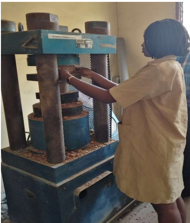
Fig. 3. Performing compression test on the brick samples
