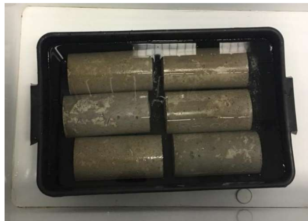
Fig. 3. Specimens submerged in water and kept in a freezer.
