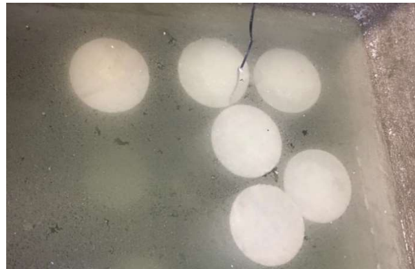
Fig. 2. Specimens submerged in water
