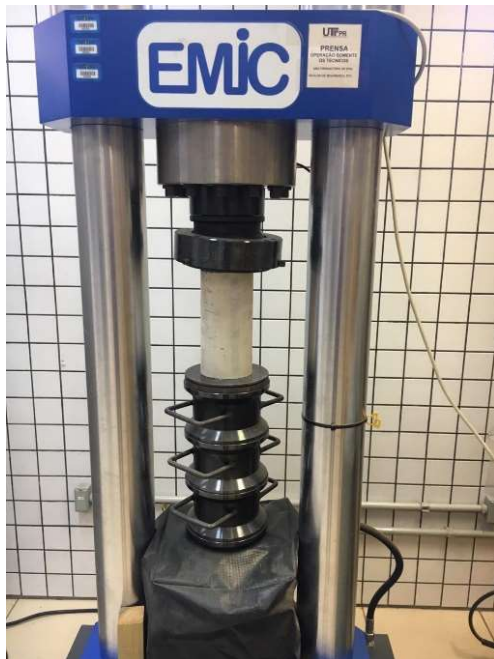
Fig. 5. Hydraulic press in which specimens were tested
