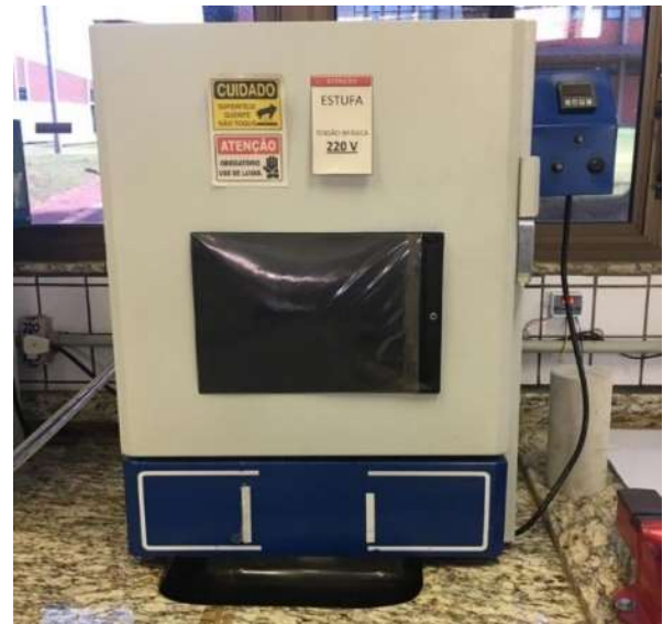
Fig. 1. Laboratory oven for curing of group 1
