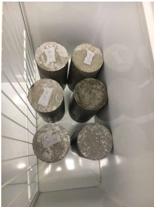
Fig. 4. Specimens cured in a freezer
