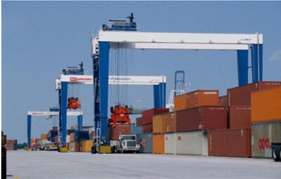
Figure 2 . A Yard Crane Interacting with a Yard Truck
