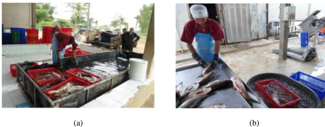
Figure 2: The chilling with ice-water slurry was implemented in the mass production of the factory for (a) preparation process (b) in the guts removal process
