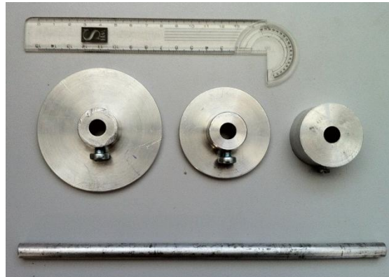
Figure 2. Model foundation system
