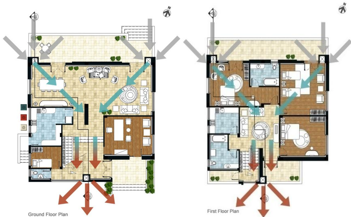
Figure 7. Natural Ventilation System (Ground & First Floor Plans)
